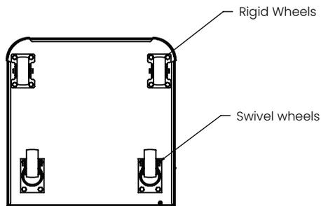
Lay the unit on its side and attach the 4 casters with the 16-- 1/4-20 hex bolts. 2 rigid wheels to the front and 2 swivel wheels to the back.
